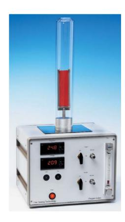
ASTM D 2863: Standard test method for measuring the minimum oxygen concentration to support candle-like combustion of plastics (oxygen index)
