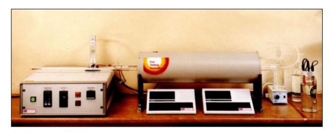
The International Electrotechnical Commission IEC 60754 Part 1 and Part 2 test is performed to determine the degree of acidity of gases evolved during the combustion of materials taken from electric cables by measuring the pH & conductivity.
