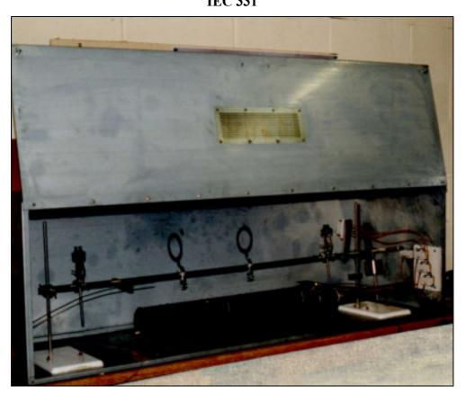
This test apparatus is for verifying the resistance to fire alone of electrical cables used for wiring and interconnection where it is required to maintain circuit integrity under fire conditions for longer periods than can be achieved with cables of conventional construction.
