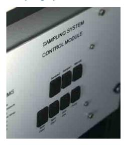
The hot-extractive sampling system consists of a heated sample gas probe, heated sample lines and heated sample pump unit. The whole system is kept at 150°C to 180°C to avoid condensation and subsequent washing of soluble fire gases out of the sample. Two-stage particle filtration is used in order to remove particles from the sample gas. The sample pump unit includes gas connections for the FTIR gas analyser:
