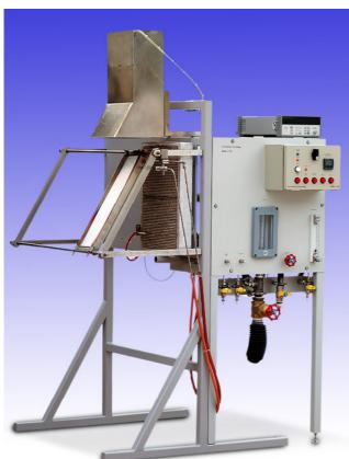
The FTT Radiant Panel Flame Spread apparatus is supplied as a complete easy-to-use system. Features include:
