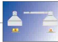
Furniture calorimeter Used to measure heat release and mass loss from furniture.
