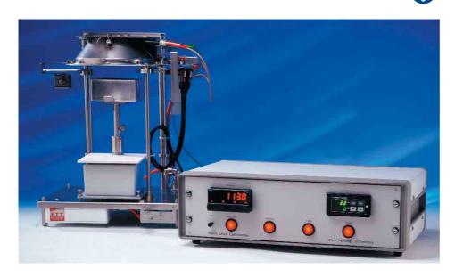
The FTT Mass Loss Calorimeter can be enhanced to be a full or partial Cone Calorimeter at any time by addition of Cone Calorimeter components. The chassis, ductwork and fans, the smoke analysis instrumentation, mass flow measurement and oxygen depletion equipment can all be added later.
