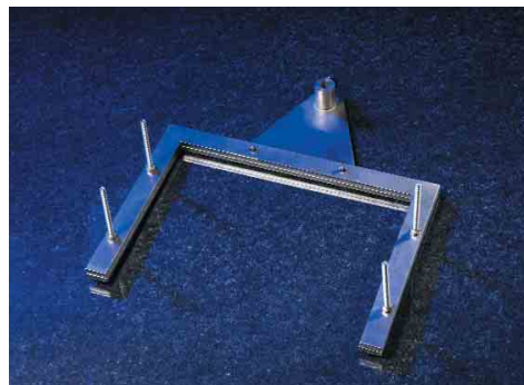
Sample holder used for products which melt or shrink away from the flame without being ignited
